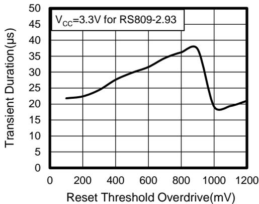
**Figure 3. Transient Duration vs Reset Threshold Overdrive**
