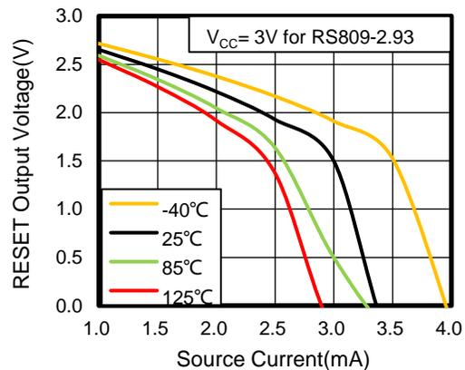
**Figure 6. RESET Output Voltage vs Source Current**
