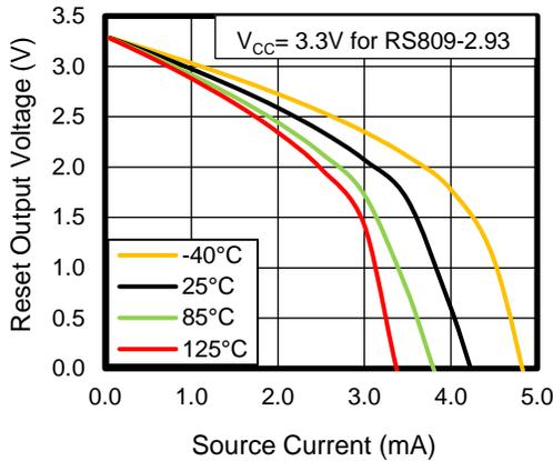
Figure 7. Reset Output Voltage vs Source Current
