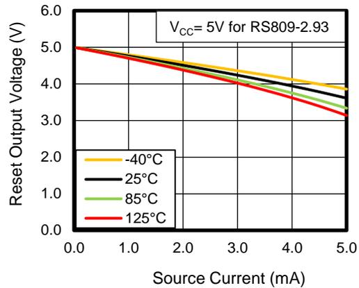
Figure 8. Reset Output Voltage vs Source Current
