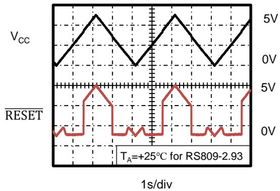
Figure 10. RESET Output Voltage vs Supply Voltage
