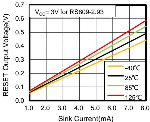
**Figure 5. RESET Output Voltage vs Sink Current**
