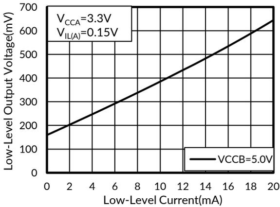
**Figure3: Low-Level Output Voltage vs Low-Level Current**
