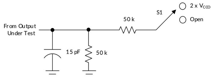
**Figure 18. Load Circuit For Enable/Disable Time Measurement**
