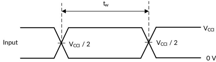
(1) All input pulses are measured one at a time, with one transition per measurement.
