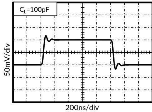
Figure 10. Small-Signal Step Response
