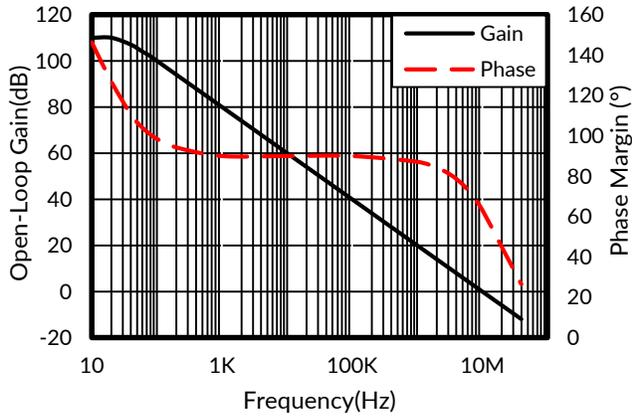
**Figure 1. Open-Loop Gain and Phase vs Frequency**
