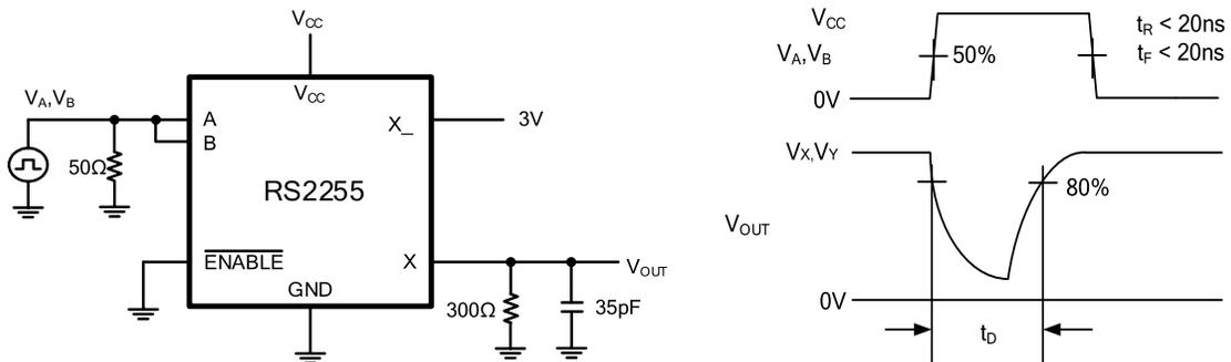
**Test Circuit 3. Break-Before-Make Time Delay ( $t_D$ )**
