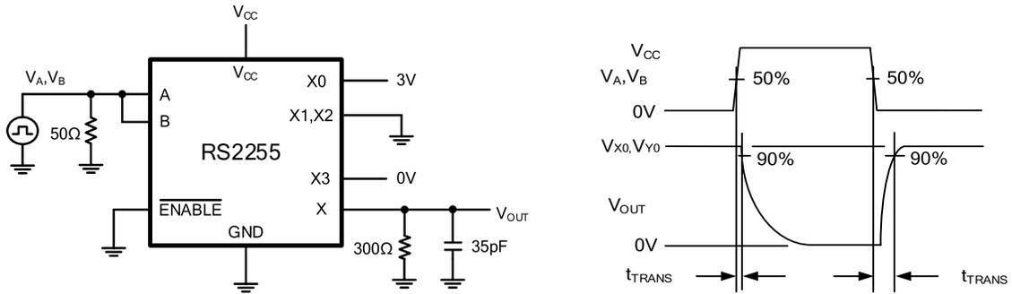
**Test Circuit 1. Address Transition Times ( $t_{TRANS}$ )**
