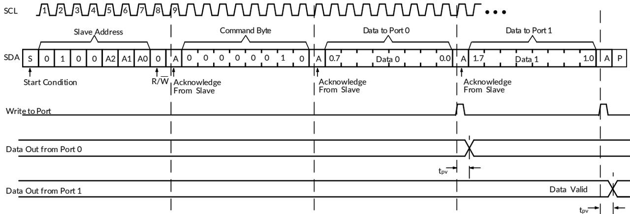
**Figure 10. Write to Output Port Registers**
