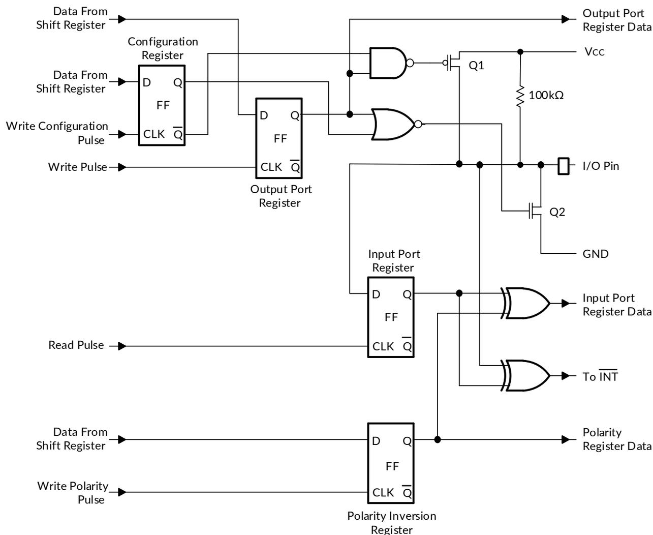
**Figure 5. Simplified Schematic of P-Port I/Os**
