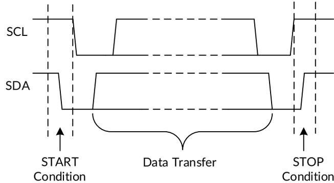
**Figure 6. Definition of Start and Stop Conditions**
