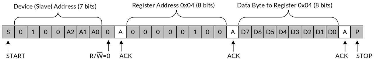
**Figure 9. Write to the Polarity Inversion Register**
