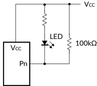
**Figure 17. High-Value Resistor in Parallel With LED**
